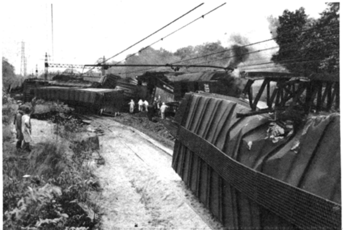
Freight train derailed in Darien due to a washout from the flood of October, 1955. Post file photo.
